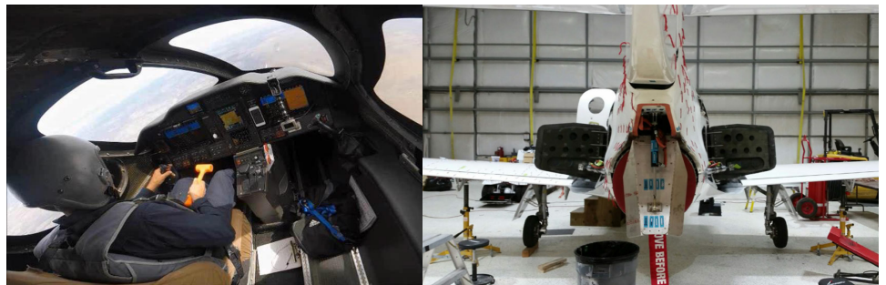
Left: Pilot performing stick and pedal rap testing with a dead blow hammer. Right: Air brakes deployed on PoC aircraft
