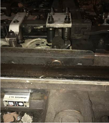
enDAQ sensor affixed track-side to monitor track vibration
