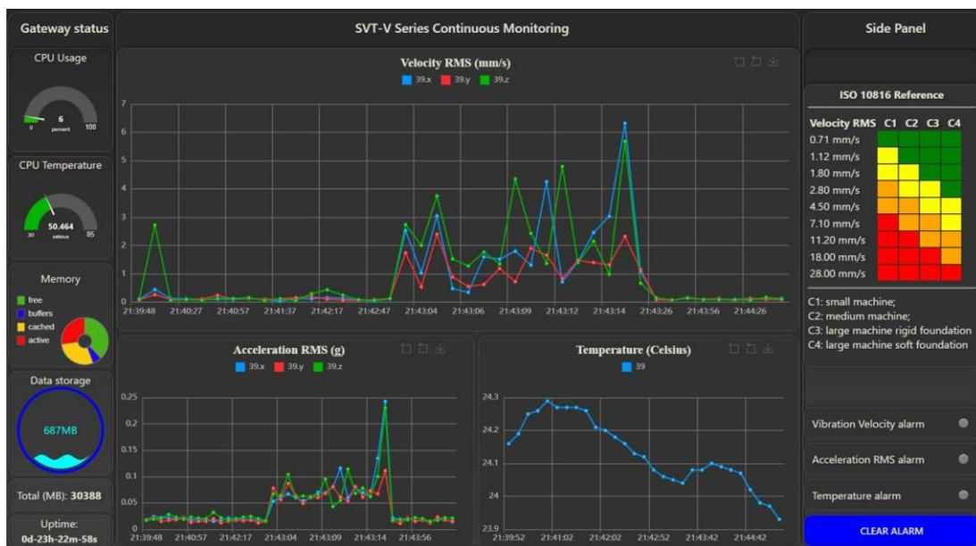
Figure 42 True real-time vibration monitoring by SVT-V sensors
