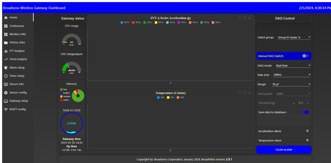
Figure 20 Standard front panel
