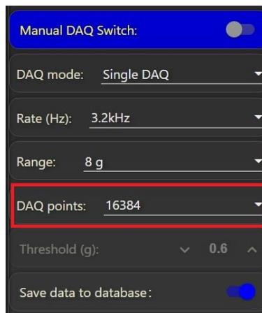
Figure 29 Single DAQ mode sample points adjustment
