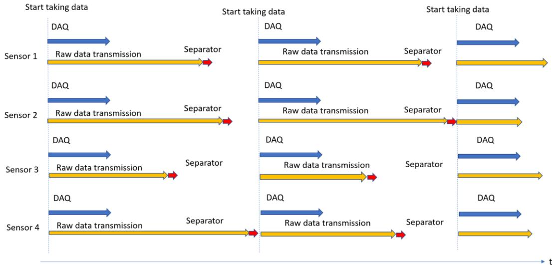
*Figure 36 Synchronized multi DAQ mode timing chart*
