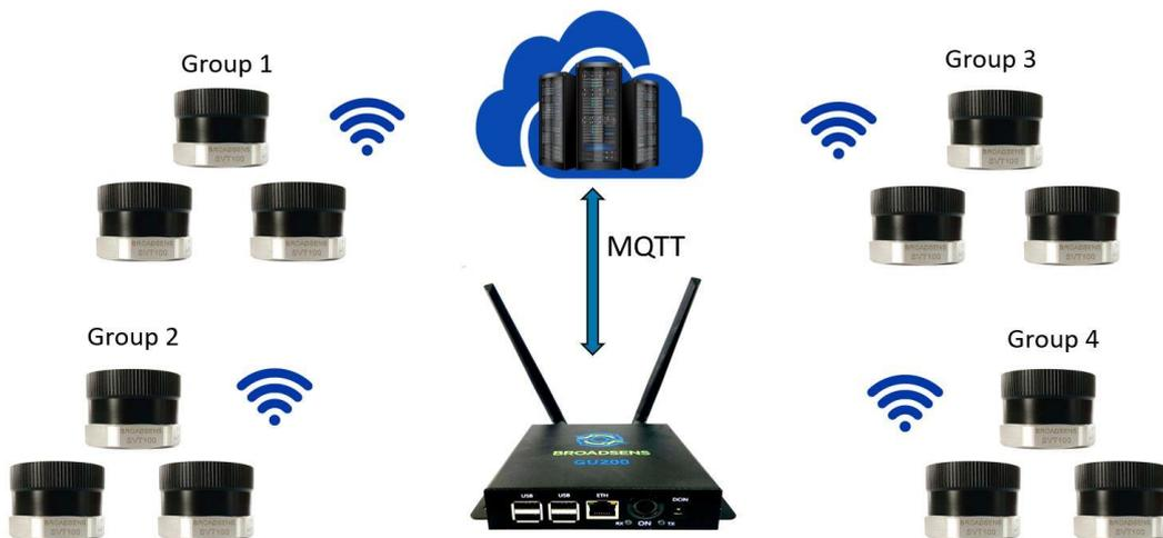
*Figure 1 Group control of multiple wireless sensors*
