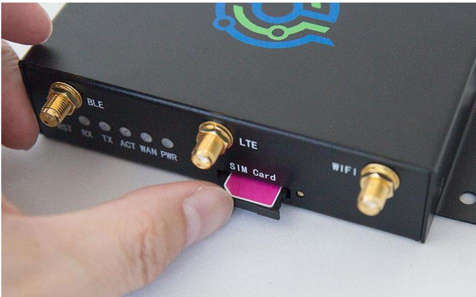
Figure 11 Insert SIM card tray to GU300S
