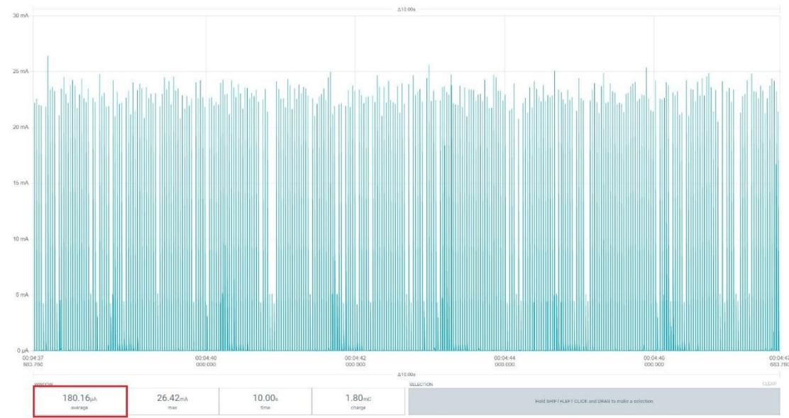
Figure 26 Power consumption of SVT-A series sensor in real-time mode 50Hz
