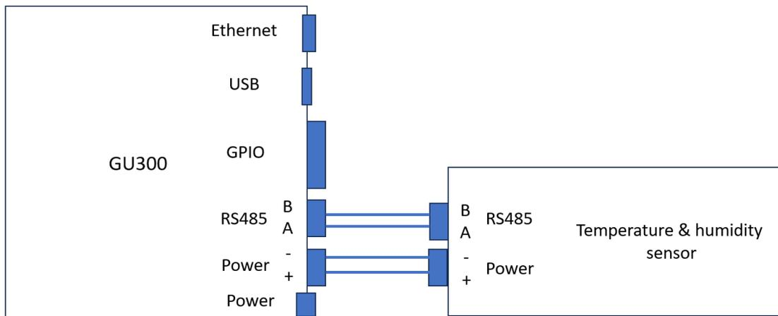
*Figure 100 Modbus RTU sensor connection with gateway*
