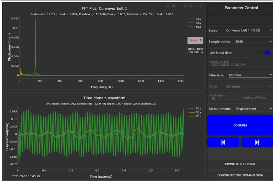
Figure 62 Displacement measurements
