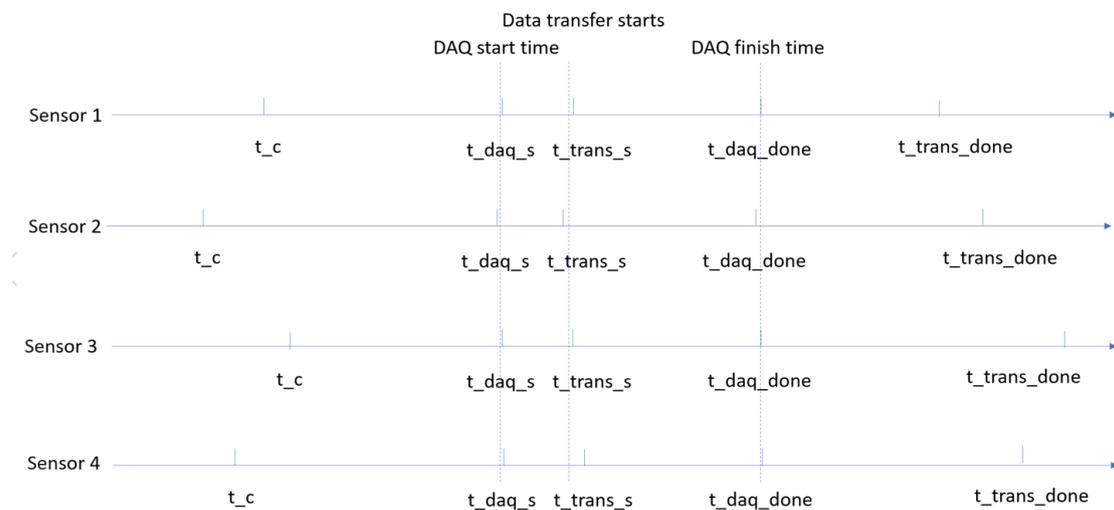
*Figure 31 Synchronized single DAQ mode timing*
