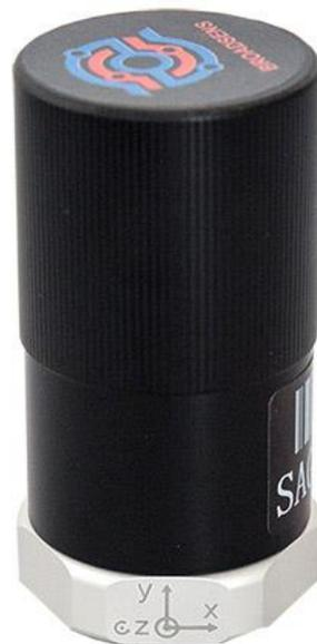
*Figure 103 SAG IMU sensor x, y, z axis*
