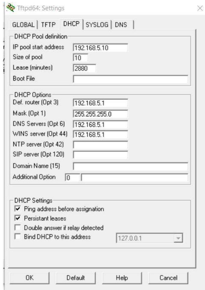
*Figure 116 Set up DHCP for Ethernet adapter*
