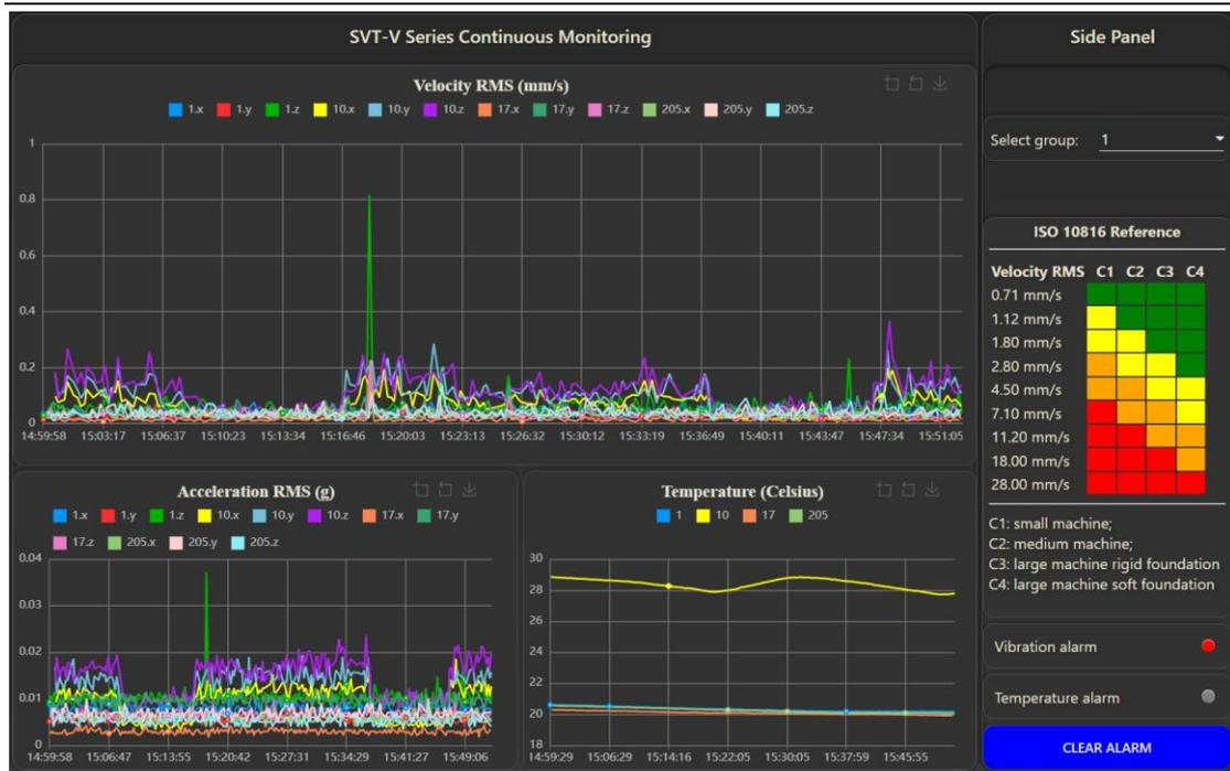
Figure 41 SVT-V sensors continuous real-time vibration monitoring
