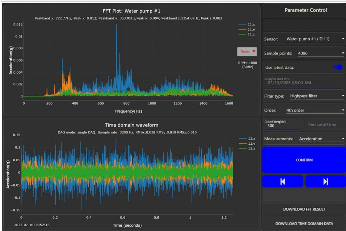
Figure 60 4<sup>th</sup> order High pass filter applied to signal
