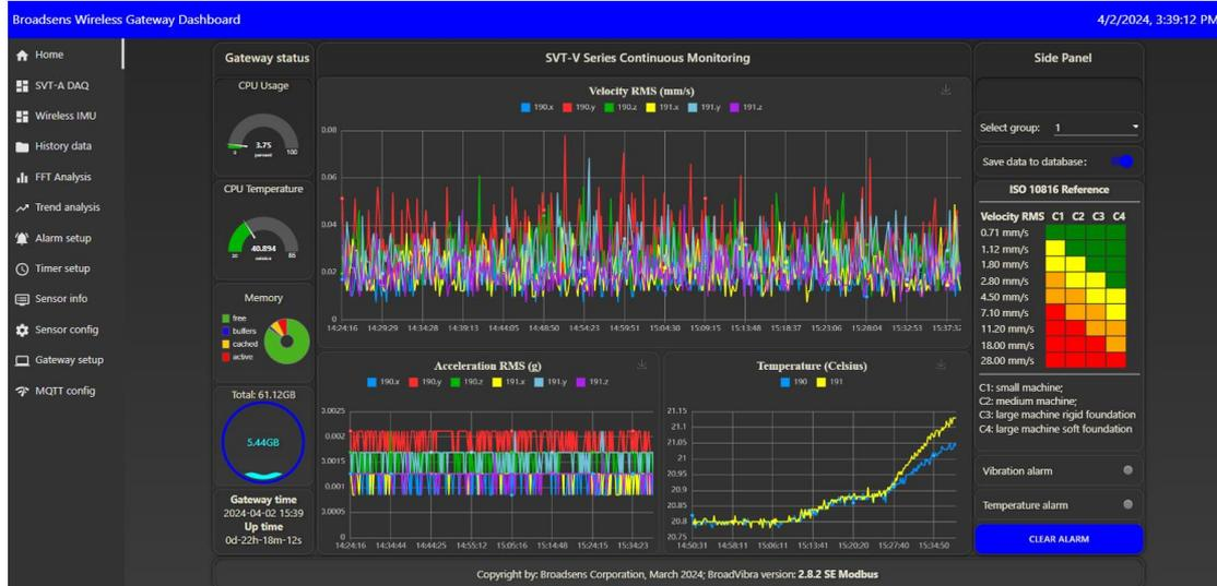
Figure 22 Special edition front panel with SVT-V sensors in homepage
