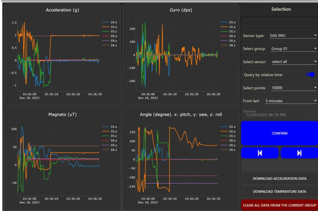
Figure 52 SAG wireless IMU sensor data review
