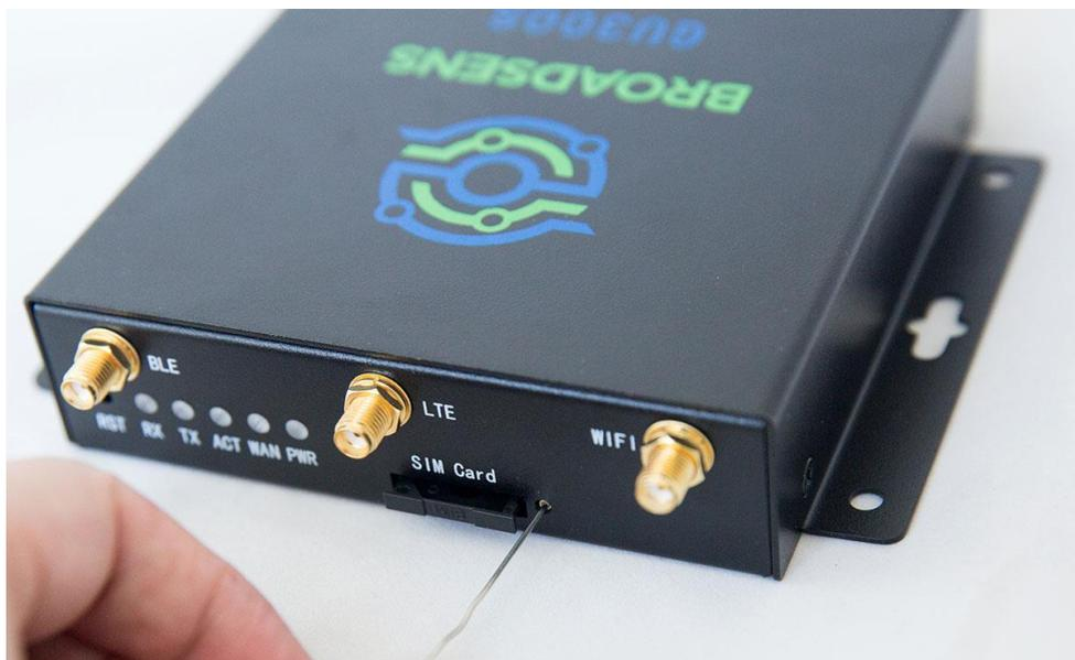
*Figure 9 Eject SIM card tray from GU300S*
