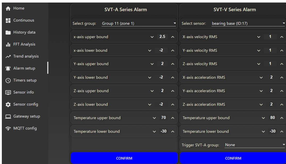
Figure 64 Alarm setup
